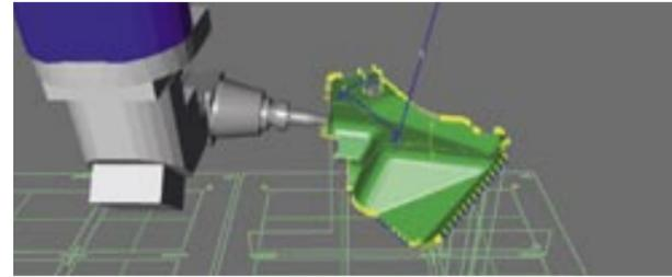
**Production simulations** | Many types of design and programming software enable users to simulate production. This allows design engineers to test sheet metal parts as often as necessary to identify problems. Today, computer simulation has become an indispensable pre-production tool, particularly for the manufacture of complex parts.
