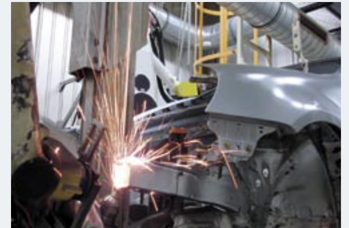
Measuring, cutting, and welding in a VW production cell
